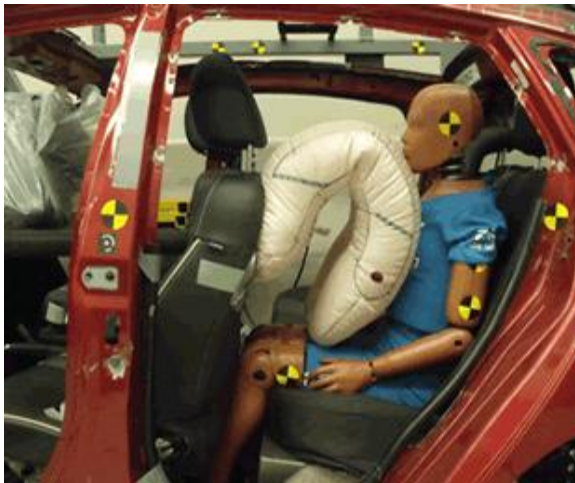
Fig 3- Roof air bag
